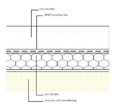
**Location: DCT GA** is laid directly onto level slab. In addition, **DCT GA** can be placed vertically around the edge of the slab inside the form-work.
