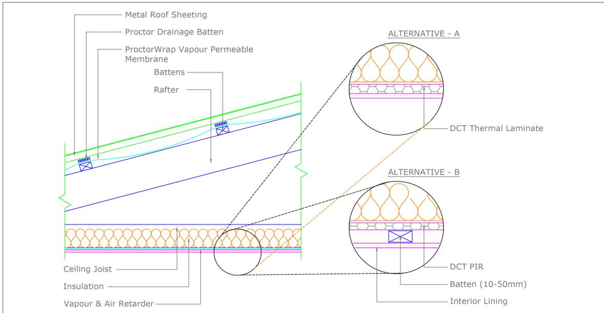
Location: Under profiled metal roofing
