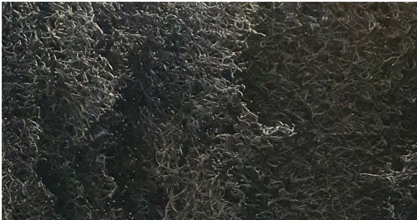
Fig 1. PP mesh left exposed far beyond the recommended allowable UV exposure period.
